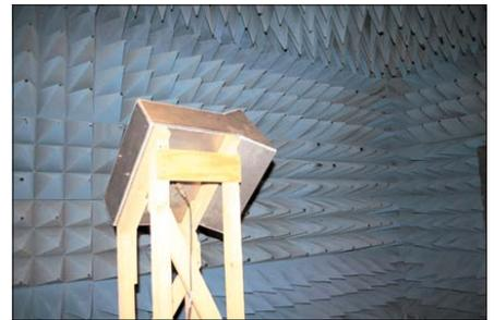
**The indoor RF anechoic chamber.**
