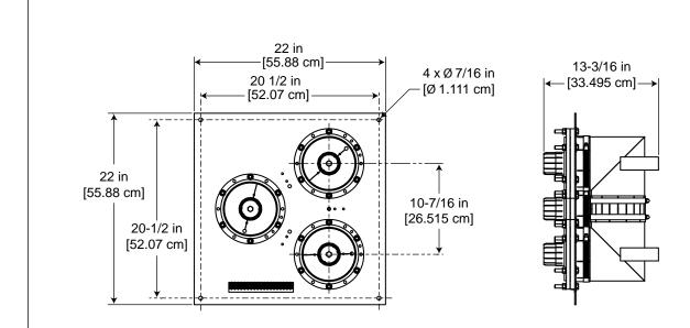
Patch Panel, 6-1/8" Flanged 3 Ports with 1 U-Link Part No. 618F-PP3
