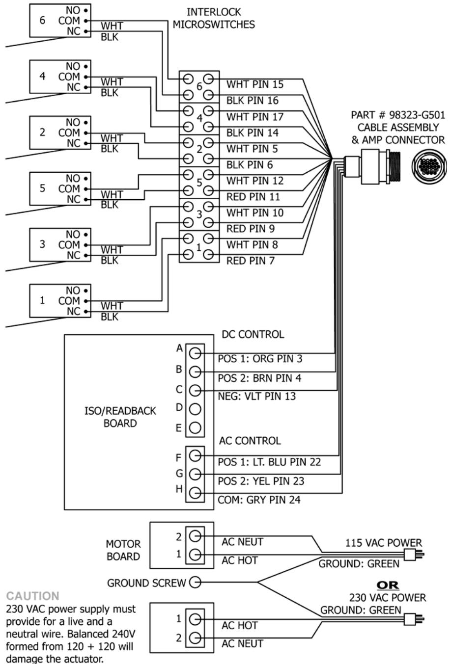
Figure 1. Electrical schematic diagram
