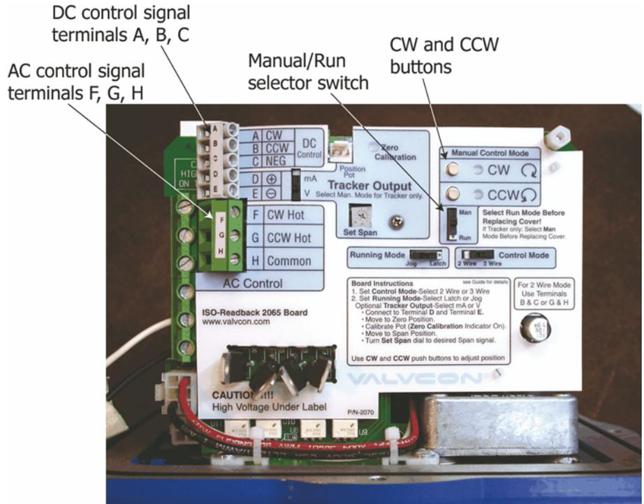
Figure 3. Connections and controls
