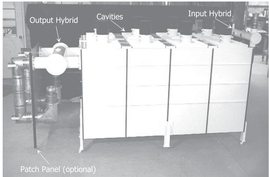
Figure 1. Typical Balanced Combiner Module, Front View
