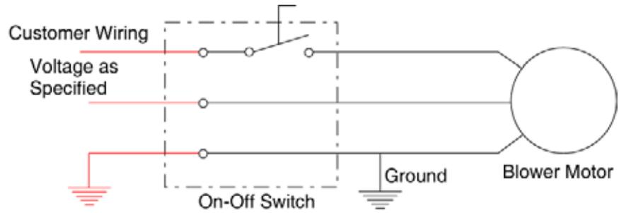
Wire to the switch inside the switch housing.
