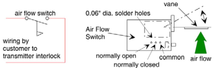
Wire directly to the switch as shown.
