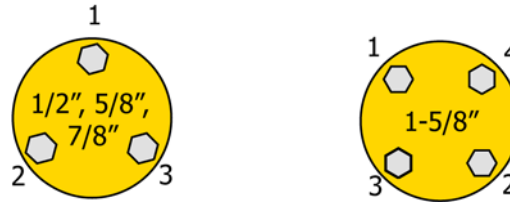
Figure 6. Flange Bolt Tightening Sequences
