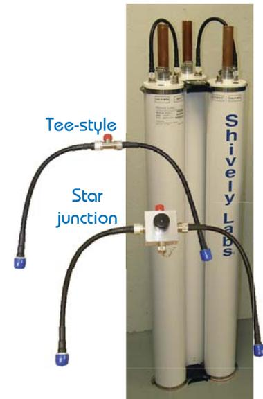
3-pole filter module and output networks
