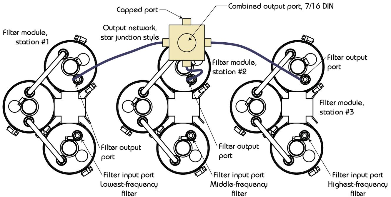
Figure 2. Typical three-station 3-pole combiner layout, top view
