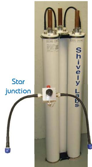
3-pole filter module and output networks
